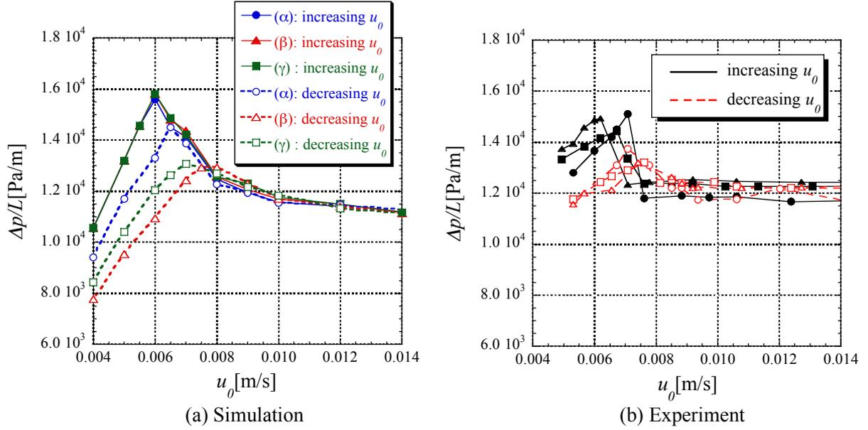
Fig. 8 Pressure gradient as a function of superficial gas velocity
