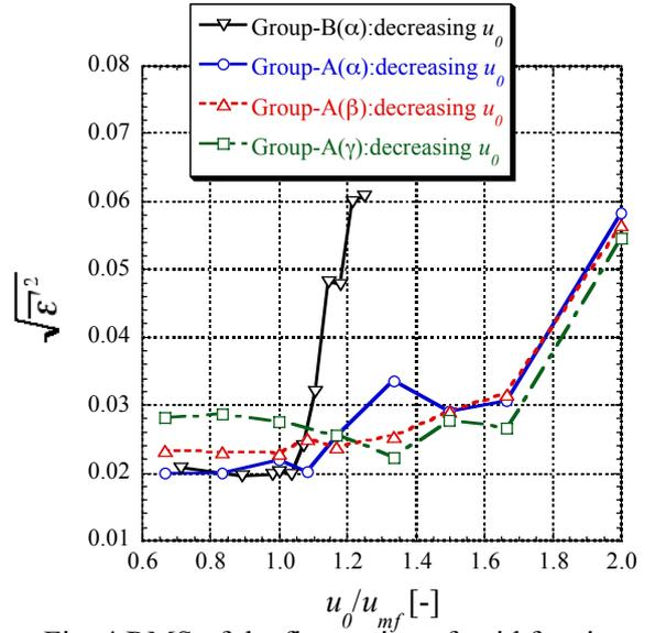
Fig. 4 RMS of the fluctuation of void fraction as a function of superficial gas velocity.
