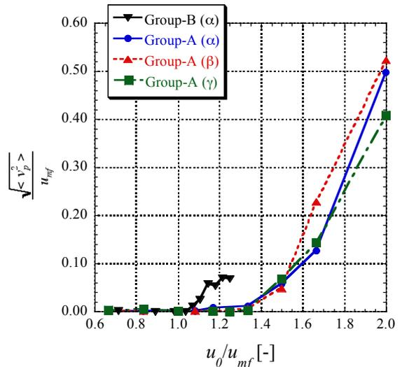
Fig. 5 RMS of particle velocity as a function of superficial gas velocity.
