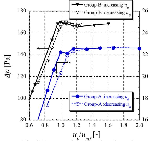
Fig. 3 Pressure drop as a function of superficial gas velocity.
