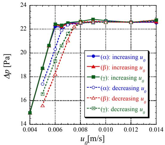
Fig. 7 Pressure drop as a function of superficial gas velocity.
