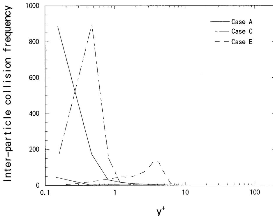
FIG. 13. Mean interparticle collision frequency distribution in wall coordinates.
