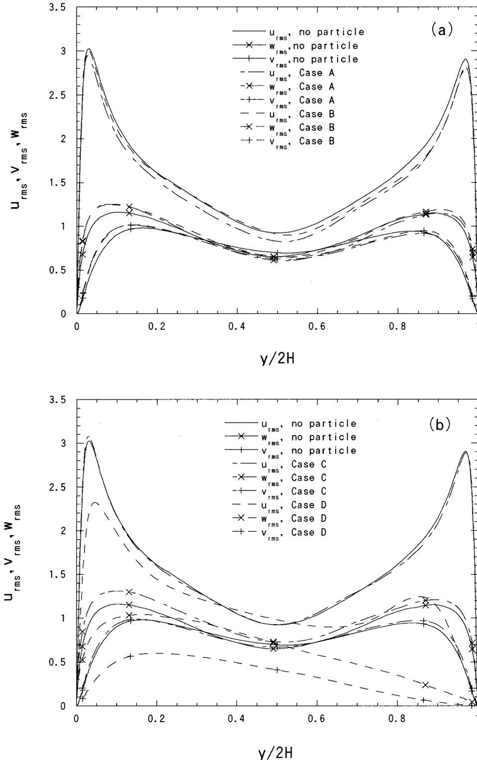
FIG. 5. Root-mean-square values of the velocity fluctuations of the fluid distribution ( $u_{rms}/u_\tau$ ,  $v_{rms}/u_\tau$ , and  $w_{rms}/u_\tau$ ) comparison among different cases in global coordinates,  $Ro = 0.075$ . (a) Cases A and B; (b) Cases C and D; (c) Cases E and F.
