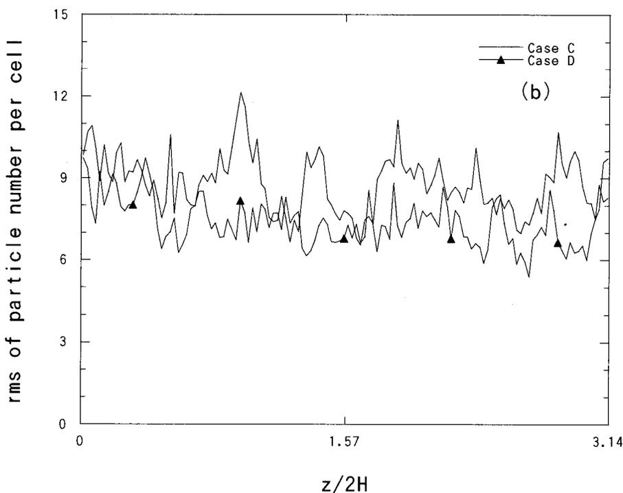
FIG. 11. Comparison of  $N_{rms}(z)$  for the particles at time  $8 H/u_\tau$ . (a) Cases A and B; (b) Cases C and D; (c) Cases E and F.
