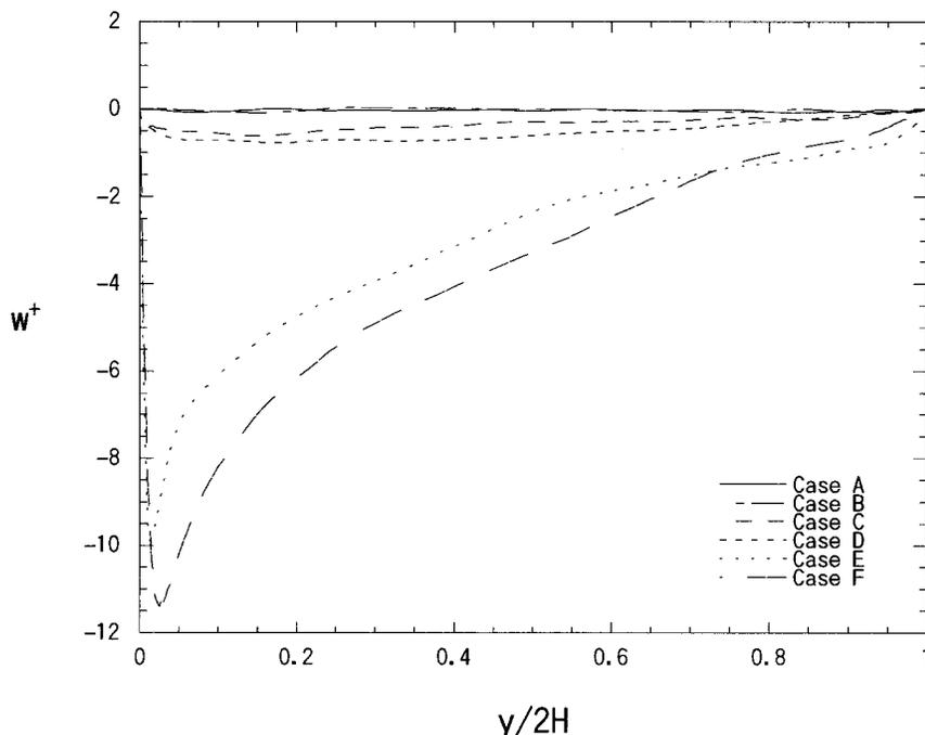
FIG. 3. Mean spanwise velocity distribution of the fluid,  $w^+$ , in global coordinates,  $Ro = 0.075$ .
