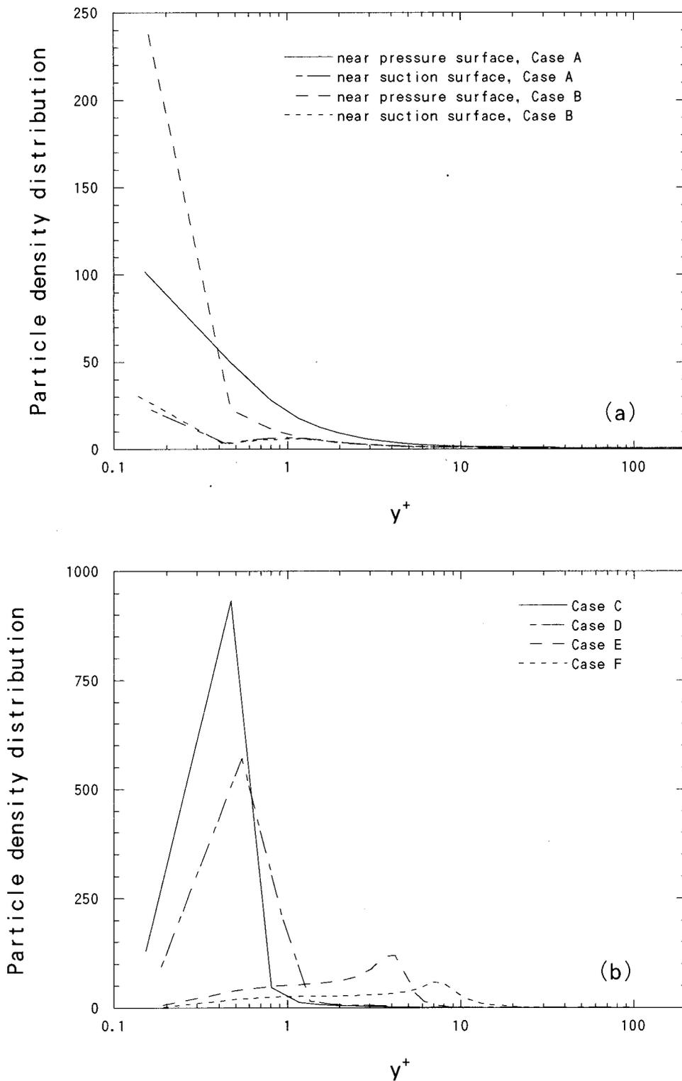
FIG. 12. Mean particle density distributions,  $\phi_{y,v}/\phi_v$ , in wall coordinates. (a) Lycopodium particles near both surfaces; (b) glass and copper particles near the pressure surface.
