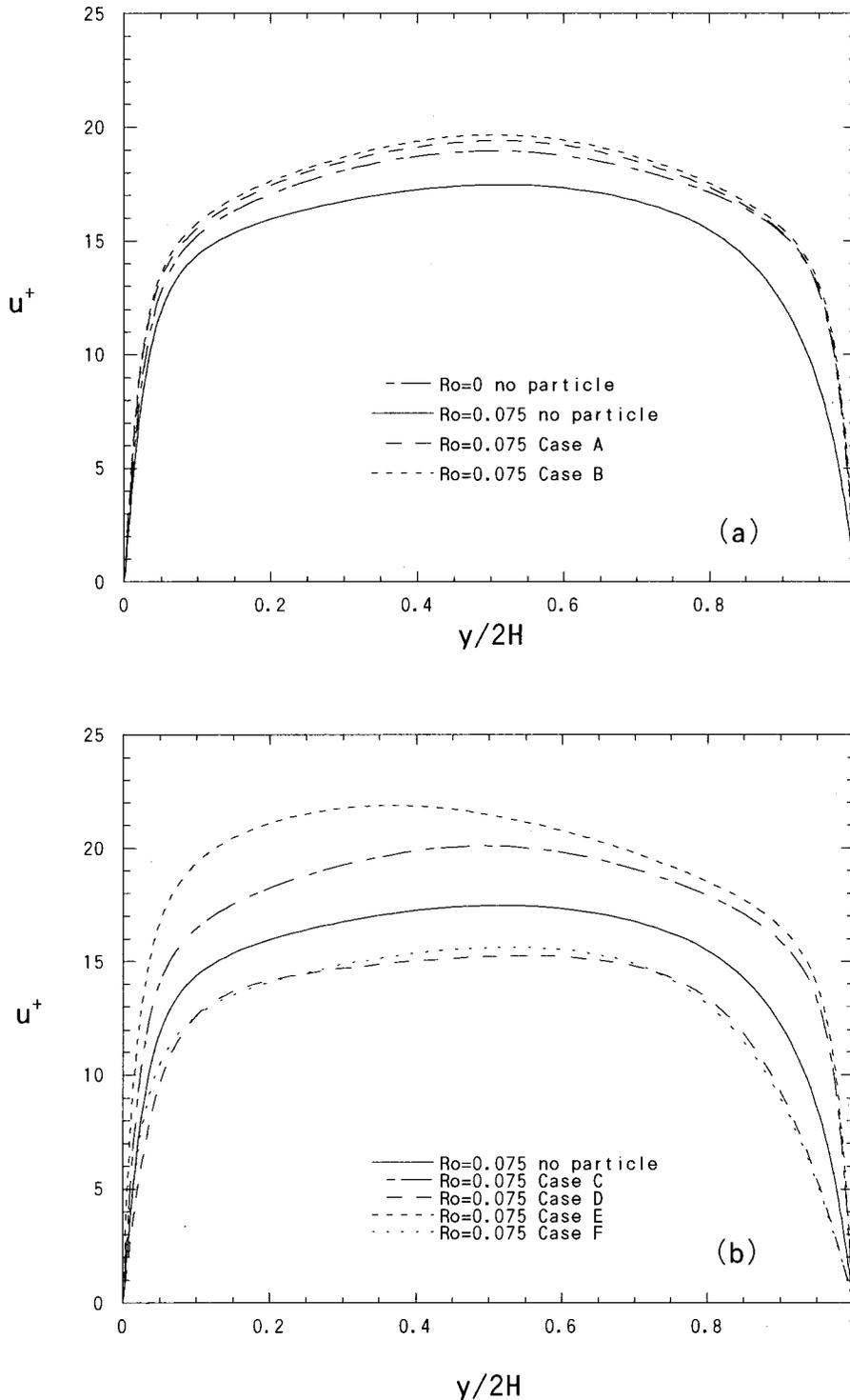
FIG. 2. Mean streamwise velocity distribution of the fluid,  $u^+$ , in global coordinates. (a) Cases A and B; (b) Cases C, D, E, and F.
