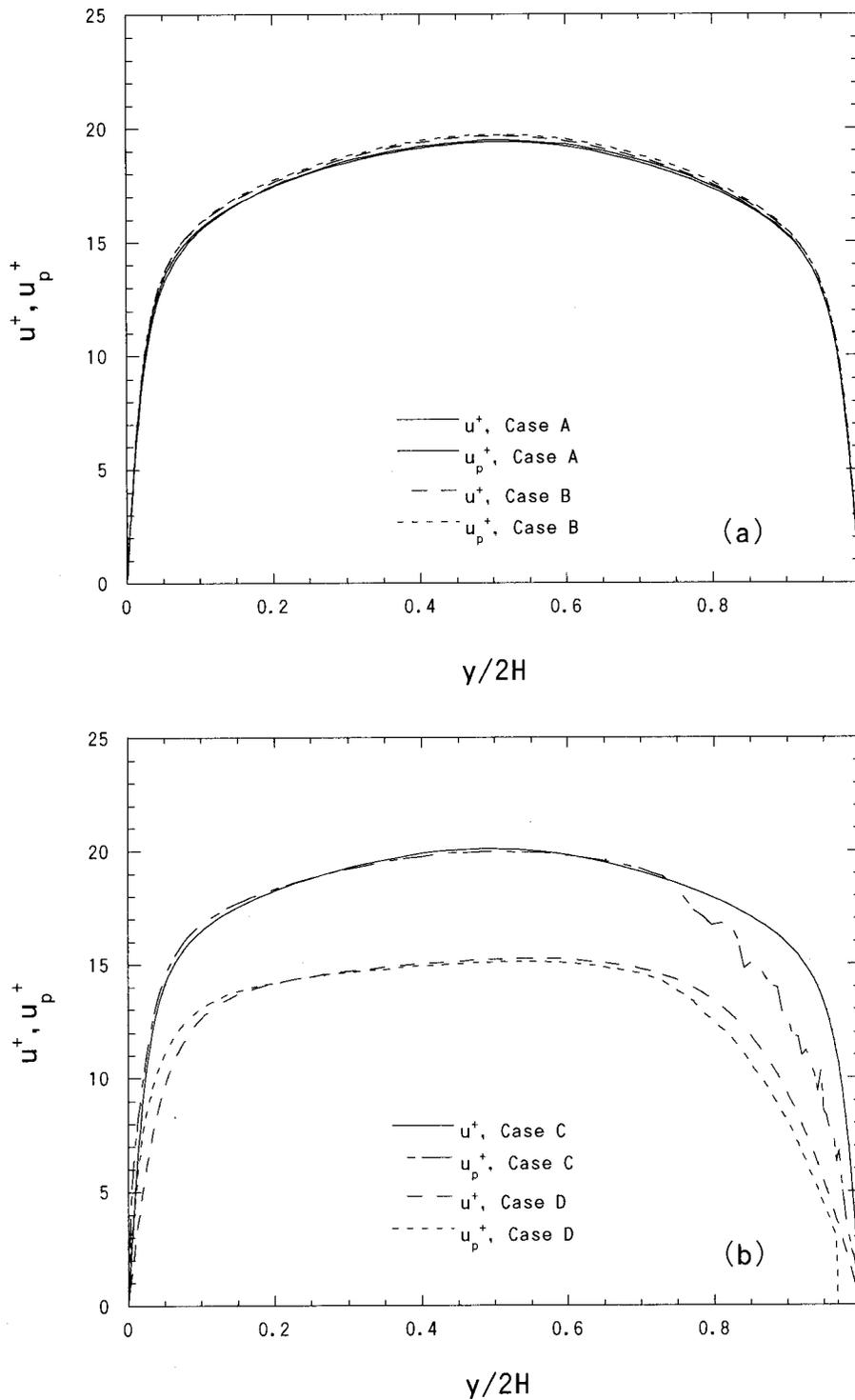
FIG. 4. Mean streamwise velocity distribution of the fluid and the particles,  $u^+$  and  $u_p^+$ , in global coordinates,  $Ro=0.075$ . (a) Cases A and B; (b) Cases C and D.
