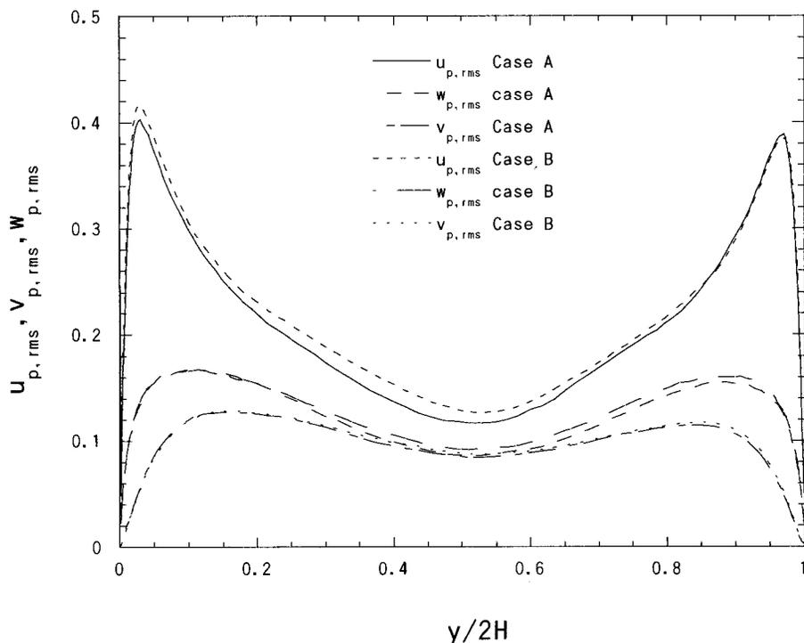
FIG. 6. Root-mean-square values of the particle velocity fluctuations distribution ( $u_{p,rms}/u_\tau$ ,  $v_{p,rms}/u_\tau$ , and  $w_{p,rms}/u_\tau$ ) comparison between case A and case B in global coordinates,  $Ro = 0.075$ .
