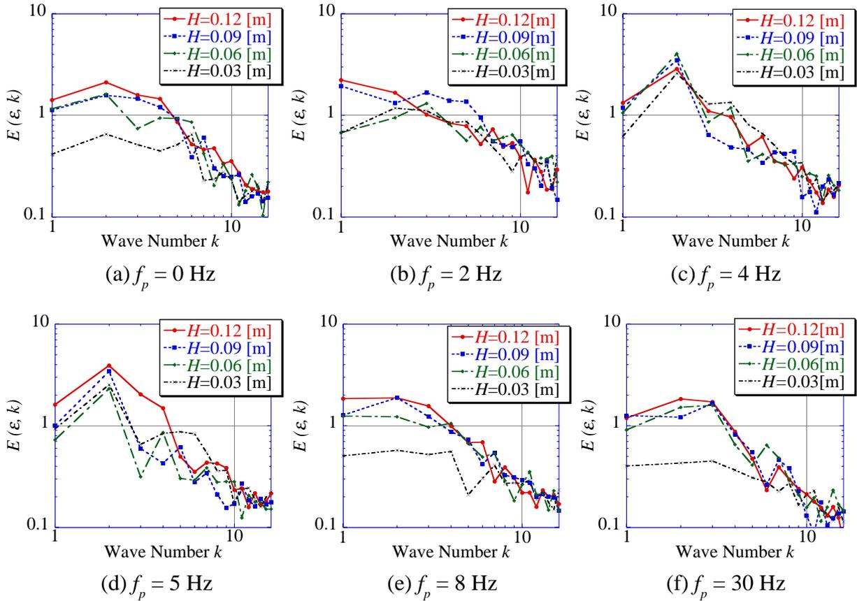
Fig. 3. Power spectrum of voidage distribution : Group B particles.
