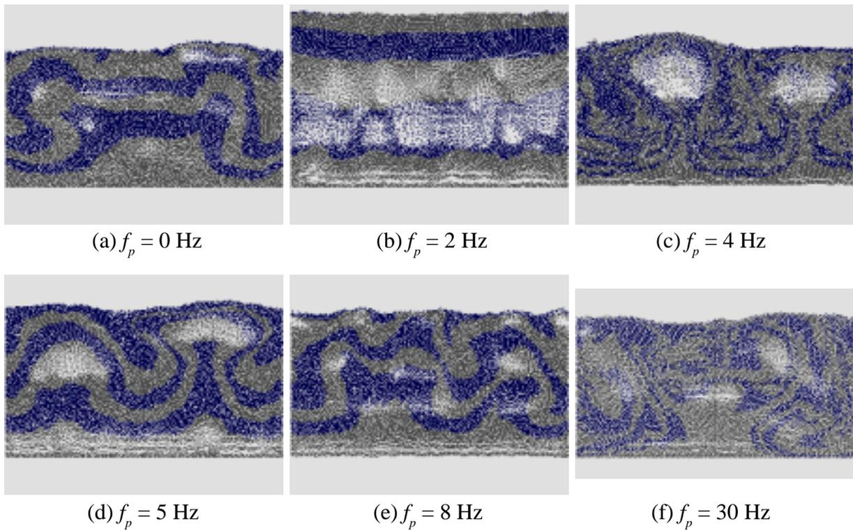
Fig. 2. Snapshot of particle motion : Group B particles.
