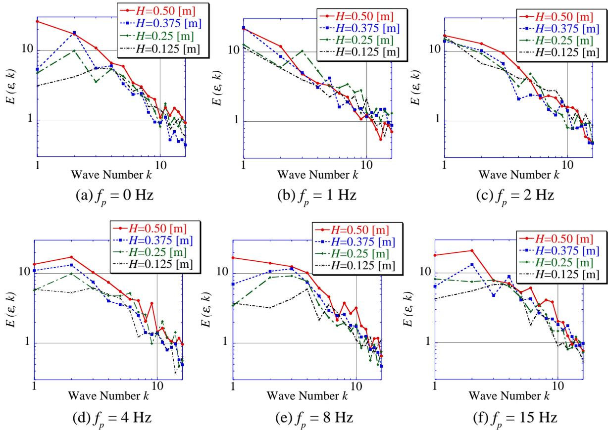
Fig. 5. Power spectrum of voidage distribution : Group D particles.
