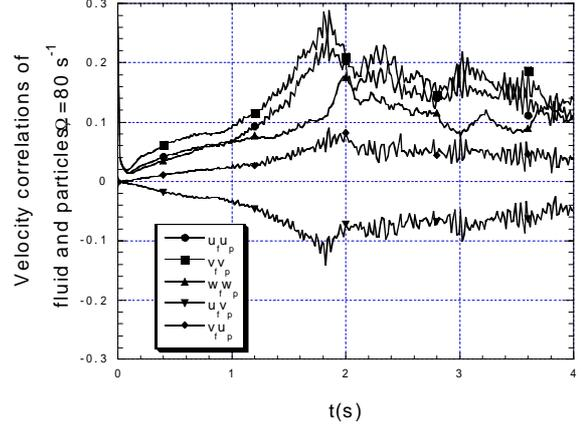
Fig.7 Time development of one-point velocity correlations between the fluid and the particles for the case with  $\Omega=80 \text{ s}^{-1}$ .
