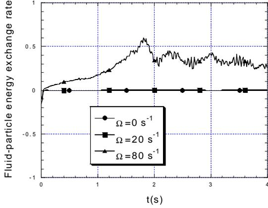
Fig.2 Evolution of fluid-particle energy exchange rate with time,  $\dot{F}$ . The dimensional unit of  $\dot{F}$  is  $m^2/s^3$ .
