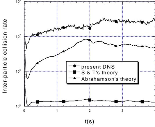
Fig.6 Comparison of the inter-particle collision rates among from the present DNS, Suffman and Turner's theory and Abrahamson's theory with time for the case with  $\Omega=80 \text{ s}^{-1}$ .
