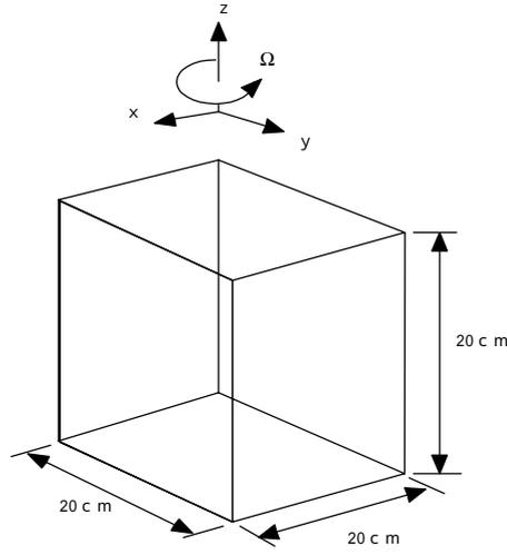
Fig. 1 Flow geometry and coordinate system
