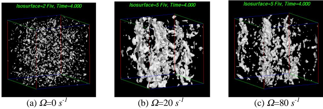
Fig. 5 Isosurfaces of particle number per cell at time  $t=4$  s
