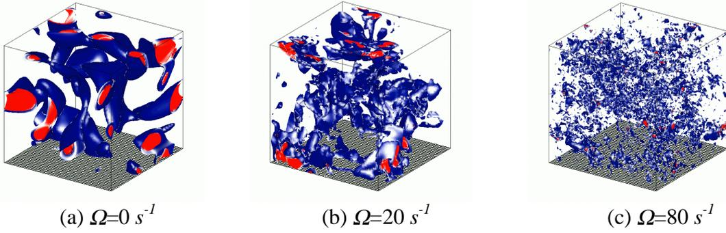
Fig. 8 Isovorticity surfaces of different cases at time  $t=4 \text{ s}$ .
