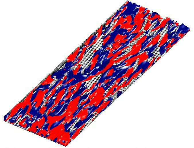
**Fig. 10 Fluid's streamwise fluctuation vorticity structure of the particle-laden flow at  $Ro=0.1$  near the pressure surface**
